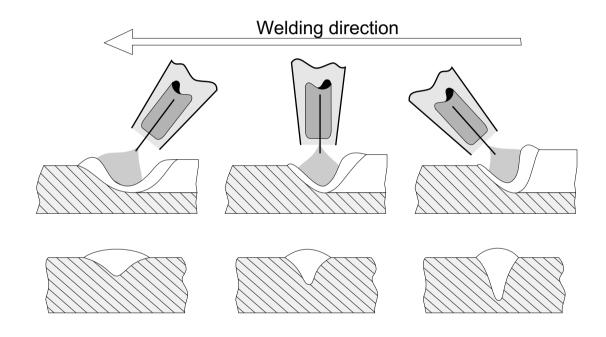
Torch positionpiercingverticaldraggingPenetrationshalloweraveragedeeperWeld widthwideraveragetighter
